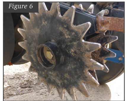
Figure 6. Spike toothed closing wheel.
